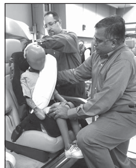
Engineers adjust a crash dummy with an inflatable seat belt on a demonstrator at Ford Motor Co. in Dearborn, Mich.
